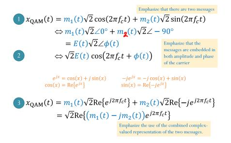
Figure 33: Three Forms of QAM
